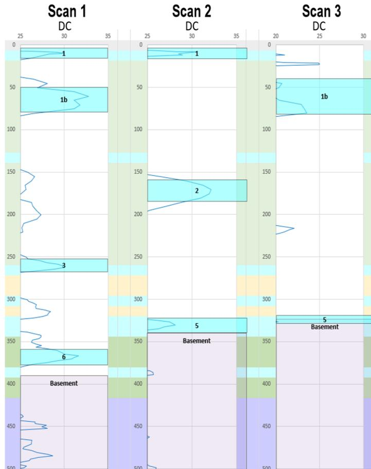
Adrok aquifer mapping using measured high DC while targeting sulfides below basement
